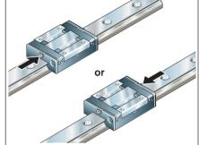
For **short-stroke** applications, apply either the total amount as per table to each end-face lube nipple, or the partial amount per side as given in the table to each side lube port.
