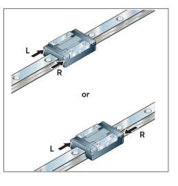
For **short stroke** applications, apply the partial amount per side as given in the table to each end-face lube port. \* (L = left, R = right)
